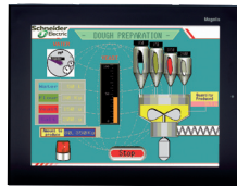
Back-lit colour TFT LCD (800 x 600 pixels)
