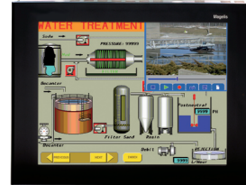
Back-lit colour TFT LCD (1024 x 768 pixels)
