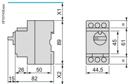
X1 Electrical clearance = 40 mm for  $U_e \leq 415$  V, or 80 mm for  $U_e = 440$  V, or 120 mm for  $U_e = 500$  and 690 V.
