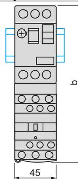
Combination GV2P + TeSys d contactor
