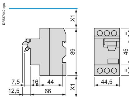
X1 Electrical clearance = 40 mm for  $U_e \leq 690$  V.
