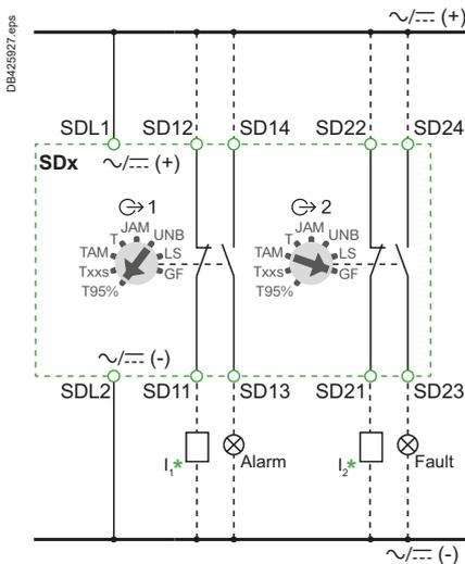
\* I1, I2: PLC digital inputs - used as alarm inputs, as an example.
